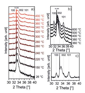
Fig. 3 Zincone calcination as followed *in situ* by XRD (a) up to 400  $^{\circ}$ C; (b) up to 600  $^{\circ}$ C with a long integration time; (c) calcined MLD-derived ZnO as measured at room temperature. Bragg peaks originating from ZnO and Si are indicated by their respective Miller indices.
