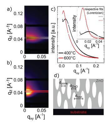
**Fig. 6** GISAXS measurement of the MLD-derived ZnO layers calcined at (a) 400 °C and (b) 600 °C; (c) interference peaks and their fitting with Lorentzian functions in order to extract the peak width  $\delta$ ; (d) a sketch of the extracted distances in the porous structures after calcination.
