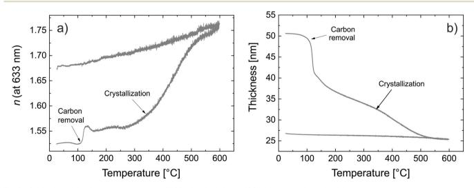
Calcination of the zincone as measured by SE (a) refractive index and (b) thickness as a function of the calcination temperature.
