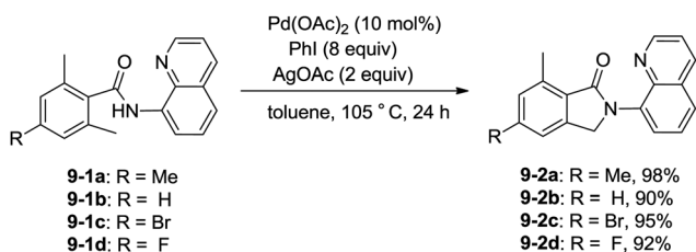
Scheme 11 Synthesis of isoindolinones with PhI.
