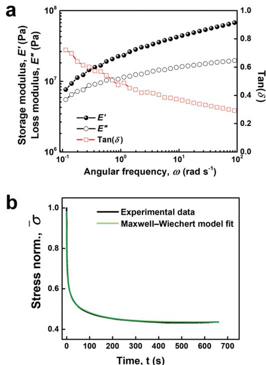
Fig. 2 Viscoelastic properties of ABA-Dopa(+) networks comparison to linear viscoelastic models. (a) Storage ( $E'$ ) and loss ( $E''$ ) modulus are plotted as a function of angular frequency obtained from tensile oscillatory sweeps ( $\epsilon = 0.5\%$ ;  $\omega = 0.1-100 \text{ rad s}^{-1}$ ). (b) Plots of stress relaxation curves for both experimental data and fitting curve using Maxwell-Wiechert model (inset).
