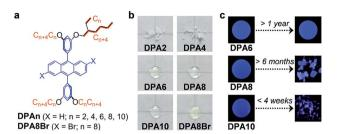
Fig. 1 (a) Chemical structures of DPAn (n=2, 4, 6, 8, and 10) and DPA8Br. (b) Photographs of freshly synthesized DPAn and DPA8Br in daylight at 20 °C, with a drop of fluid or powder of solid on a glass plate. (c) Photographs of DPA6, DPA8, and DPA10 as fresh (left) and after long-term of aging at ambient temperature (right) taken under irradiation of a UV lamp (365 nm).
