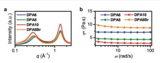
Fig. 3 (a) SWAXS profiles and (b) complex viscosity ( $\eta^*$ ) of DPA6 (blue), DPA8 (green), DPA10 (red), and DPA8Br (orange) at 30 °C (ω, angular frequency).
