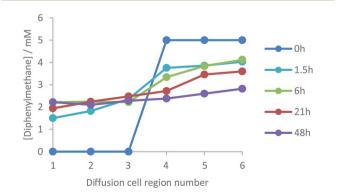
Fig. 6 Concentration profiles of diphenylmethane between regions 1 and 6 of the diffusion cell. At the start of the experiment, diphenylmethane is loaded in regions 4–6 of the cell. The points in these graphs are joined together solely as a guide to the eye.
