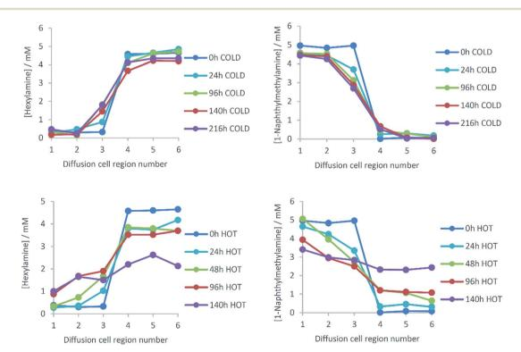
Fig. 7 Concentration profiles of (left) hexylamine and (right) 1-naphthylmethylamine between regions 1 and 6 of the diffusion cell at temperatures of (top) 5  $^{\circ}$ C and (bottom) 45  $^{\circ}$ C demonstrating the very significant impact of temperature on diffusion kinetics. At the start of the experiment, hexylamine is loaded in regions 4–6 of the diffusion cell and 1-naphthylmethylamine is loaded in regions 1–3. The points in these graphs are joined together solely as a guide to the eye.
