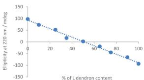
Fig. 9 (Top) CD spectra of mixtures of L-Lys-HexGel and D-Lys-HexGel at a total concentration of 5 mM in methylcyclohexane/dioxane (95/5), (Bottom) ellipticity at 220 nm extracted from the CD spectra and plotted against the % enantiomer content, demonstrating an approximately linear relationship between CD ellipticity and composition of enantiomers.
