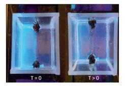
Fig. 3 Diffusion cell under UV illumination with L-Lys-NaphGel (5 mM) loaded in the left-hand side of the cell and L-Lys-HexGel (5 mM) loaded in the right-hand side of the cell – the cell is shown at the start of the experiment (left) and after some time has elapsed – supportive of the view that diffusion and amine exchange is taking place.
