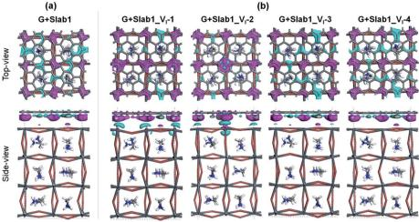
Fig. 7 Electron density difference of the (a) defect-free and (b) V<sub>1</sub>-containing graphene + MAPbI<sub>3</sub> hybrids (isovalue: 0.003 a.u.). Purple and cyan represent accumulation and depletion of electrons, respectively.
