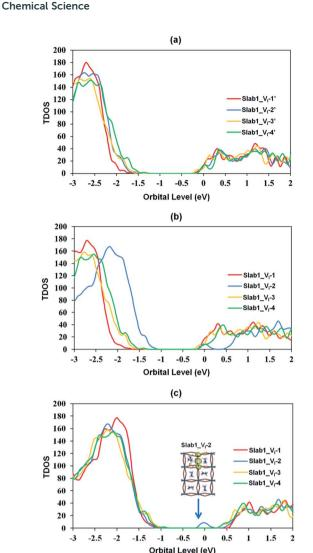
Fig. 4 Calculated total density of states (TDOS) of the  $V_1$ -containing MAPbl $_3$  slab models (a) before geometry optimization, (b) after geometry optimization, and (c) after geometry optimization where the valence band tops of all the defective slab models were adjusted to the same level. The inset in (c) indicates the orbital shape.
