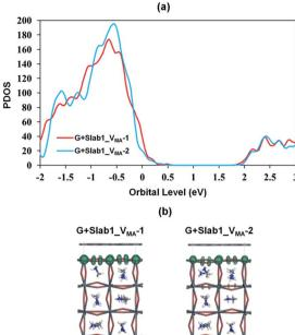
Fig. 18 (a) Calculated partial density of states (PDOS) of MAPbl<sub>3</sub> in the  $V_{MA}$ -containing graphene + MAPbl<sub>3</sub> hybrids, and (b) the orbital shape of the valence band edges of MAPbl<sub>3</sub> (isovalue: 0.015 a.u.).
