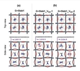
Fig. 17 (a) Defect-free and (b) V<sub>MA</sub>-containing defective graphene + MAPbl<sub>3</sub> hybrids.
