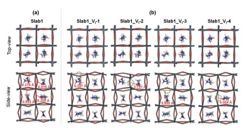
Fig. 2 (a) Defect-free and (b)  $V_1$ -containing defective MAPbI<sub>3</sub> slabs. The dashed circles indicate the position of the  $V_1$ . Each number in (b) indicates the Pb-Pb distance around the  $V_1$ .
