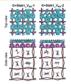
Fig. 19 Electron density difference of the  $V_{MA}$ -containing graphene + MAPbl<sub>3</sub> hybrids (isovalue: 0.003 a.u.). Purple and cyan represent accumulation and depletion of electrons, respectively.
