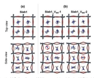
Fig. 15 (a) Defect-free and (b) V<sub>MA</sub>-containing defective MAPbl<sub>3</sub> slabs.
