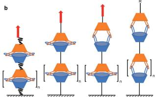
Scheme 7 AFM experiment probing the 16 hydrogen bonds uniting interlocked calix[4] arenes dimeric capsules. Red arrows indicate the direction of the force.
