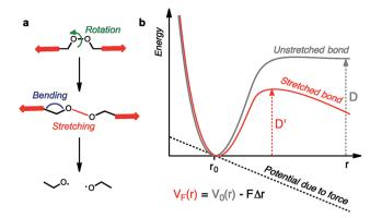
Fig. 2 Molecules under tension can undergo a series of deformations before the rupture of the weakest bond (a). The potential energy surface of a bond under tension can be described by a force-modified Morse potential (b).
