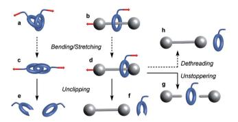
Fig. 3 Examples of mechanochemical behaviors observed in a catenane (a) and a rotaxane (b). Elongation of these mechanical bonds (c and d) can lead to their disassembly *via* the rupture of a covalent bond in the macrocycle (e and f) or the thread (g). Rotaxanes can also dissociate by dethreading (h). Plain and dashed arrows denote events involving the rupture or not of a covalent bond respectively.
