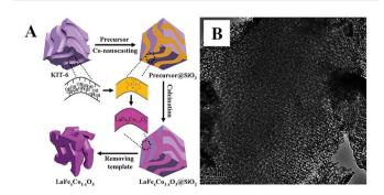
Fig. 1 (A) Synthesis process of the mesoporous  $LaFe_xCo_{1-x}O_3$  perovskite oxides by co-nanocasting process using mesoporous KIT-6 as a hard template, (B) the as-prepared mesoporous  $LaFeO_3$ . Reproduced with permission from ref. 34. Copyright© 2013, Royal Society of Chemistry.
