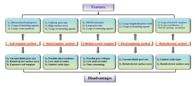
Fig. 4 Summary of synthesis methods for nanoporous perovskite metal oxides.
