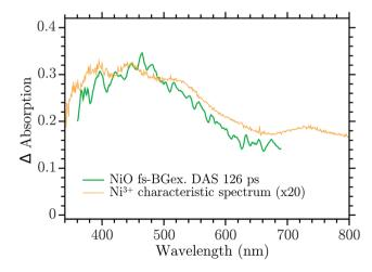
Fig. 7 Comparison between the 126 ps component of the DAS in the  $\mathrm{Ni}^{3+}$  characteristic spectrum found in ref. 24.
