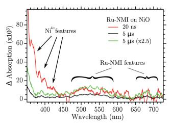
Fig. 9 Transient absorption of Ru-NMI sensitized on NiO and excited at 460 nm. The green trace is the 5  $\mu s$  trace normalized to the 20 ns one at 500 nm.
