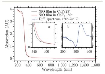
Fig. 3 Absorption spectrum of NiO on CaF $_2$  recorded at two temperatures 25 °C (black) and 180 °C (red). Inset (a) Enlargement in the 300–400 nm range. Inset (b) Spectral difference of the absorption spectrum of NiO at two temperatures (180° and 25 °C).
