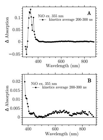
Fig. 2 Transient absorption spectra at 200-300 ns after band-gap excitation of NiO on  $CaF_2$  windows. (A) Full spectrum; (B) 350-900 nm zoom.
