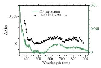
Fig. 4 Comparison between the TA at 200 ns after BG excitation and the "Ni<sup>4+</sup>" characteristic spectrum from ref. 24.
