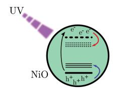
Fig. 1 Scheme of band gap excitation. The red arrow indicates a movement of an electron and the blue one indicates the movement of a hole.
