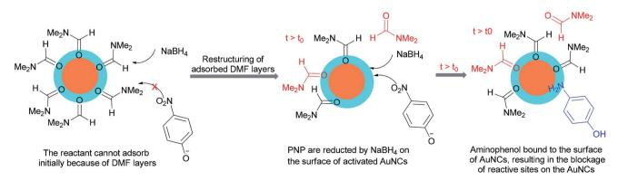
Fig. 2 Proposed mechanism for AuNC-catalyzed reduction of 4-nitrophenol to 4-aminophenol.
