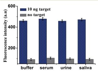
Fig. 6 Fluorescence intensity of the sensor for the detection of VEGF<sub>165</sub> in buffer and blank biological samples (human serum, urine and saliva, respectively). Error bars: SD, n=3.
