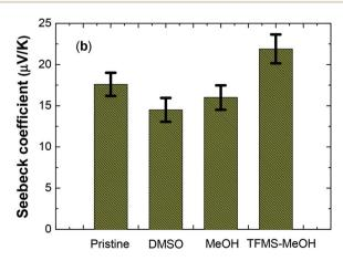
Fig. 2 Electrical conductivity (a) and Seebeck coefficient (b) of PEDOT:PSS thin films with different solvent treatment.
