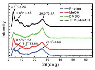
Fig. 5 X-ray diffraction (XRD) patterns of PEDOT:PSS thin films pristine and with different solvent treatment.
