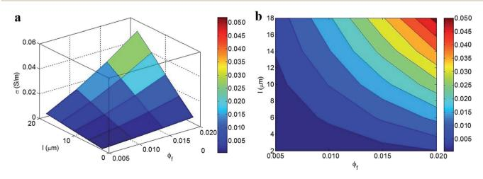
Fig. 3 (a) 3D and (b) contour patterns for the influences of " $\phi_i$ " and "l" parameters on the conductivity of nanocomposites at average levels of other variables.
