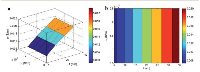
Fig. 5 The roles of "t" and " $\sigma_t$ " in the conductivity of nanocomposites by the developed model at average values of other parameters: (a) 3D and (b) contour designs.
