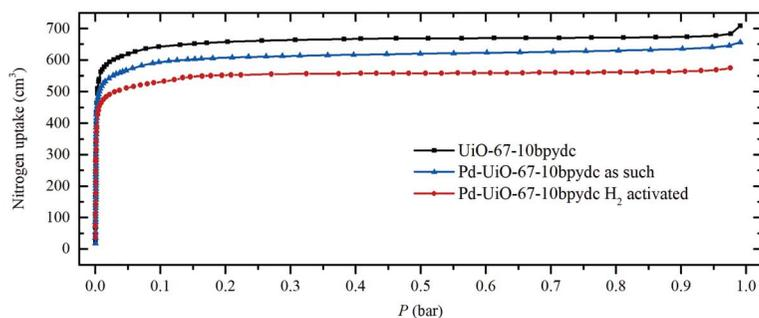
Fig. 11 N<sub>2</sub> adsorption isotherms of UiO-67 with 10% of modified ligands non-functionalized (black squares) and functionalized by Pd before (blue triangles) and after (red circles) activation in H<sub>2</sub> at 300 °C.
