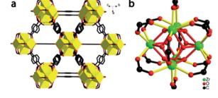
Fig. 1 Structure of UiO-66. (a) Extended 3D structure, showing the bridging terephthalates ligated to zirconia clusters. (b) Coordination geometry around the  $\rm Zr_6O_4(OH)_4(O_2CR)_{12}$  clusters.
