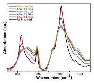
Fig. 3 FT-IR spectra of UiO-66 over the range of  $1650-1250~{\rm cm}^{-1}$  after compression and release. All absorbances were normalized to the peak at  $1019~{\rm cm}^{-1}$  (cf. ESI Fig. S4†).
