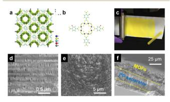
Fig. 1 MOF-decorated separator. (a) Illustration of the structure of NH<sub>2</sub>-MIL-125(Ti). (b) One node of the MOF structure. (c) MOF film coated on PP separator membrane. (d) Top-view SEM image of the pristine separator. (e) Top-view SEM image of the MOF-decorated separator. (f) Cross-sectional view of MOF-decorated separator.
