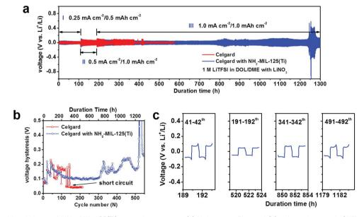
Fig. 3 Li|Li cells with pristine and NH $_2$ -MIL-125(Ti)-coated separators. (a) Voltage profiles and (b) voltage hysteresis (difference between the voltage of Li stripping and that of Li plating) of Li metal plating/striping in symmetric Li|Li cells with pristine and NH $_2$ -MIL-125(Ti)-coated separators. (c) Voltage profiles for specific cycles of the Li|Li cell with the NH $_2$ -MIL-125(Ti)-coated separator. The electrolyte is 1 M LiTFSI in DOL/DME with 2% LiNO $_3$  additive.
