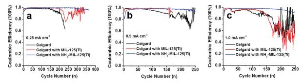
Fig. 5 Electrochemical performance of Li|Cu cells with pristine, MIL-125(Ti)-coated and NH<sub>2</sub>-MIL-125(Ti)-coated separators at various current densities. CE of Li plating/stripping at (a) 0.25, (b) 0.5 and (c) 1.0 mA cm<sup>-2</sup>, with a cut-off capacity of 1.0 mA h cm<sup>-2</sup>. Electrolyte used is 1 M LiTFSI in DOL/DME with 2% LiNO<sub>3</sub> additive.
