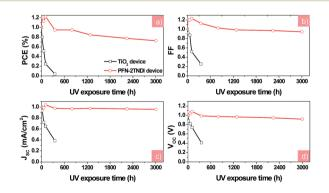
Fig. 5 The evolution of solar cell parameters (normalized (a):  $V_{\rm OC}$ , (b):  $J_{\rm SC}$ , (c): FF, (d): PCE) as a function of testing time under UV illumination for the PFN-2TNDI- and TiO<sub>2</sub>-based perovskite solar cells. The devices were stored under exposure to UV in a N<sub>2</sub>-filled glove-box during testing.
