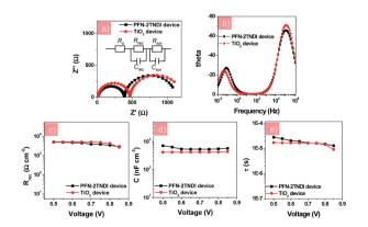
Fig. 4 (a) Nyquist plots and (b) Bode plots of perovskite solar cells with different electron transport layers; (c) the recombination resistance  $R_{\text{rec}}$ ; (d) the capacitance (C) and (e) recombination lifetime ( $\tau$ ) derived from the high frequency region as a function of the applied voltage.
