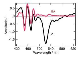
Fig. 5 Modeled electroabsorption signal of a suspension of  $CH_3$ - $NH_3PbBr_3$  nanoparticles in chlorobenzene. The blue part of the observed transient absorption spectrum measured at a time delay of 2 ps (black line) fits well with a simulated electroabsorption spectrum (red) dominated by the second derivative component of the ground state absorption spectrum (see ESI† for details).
