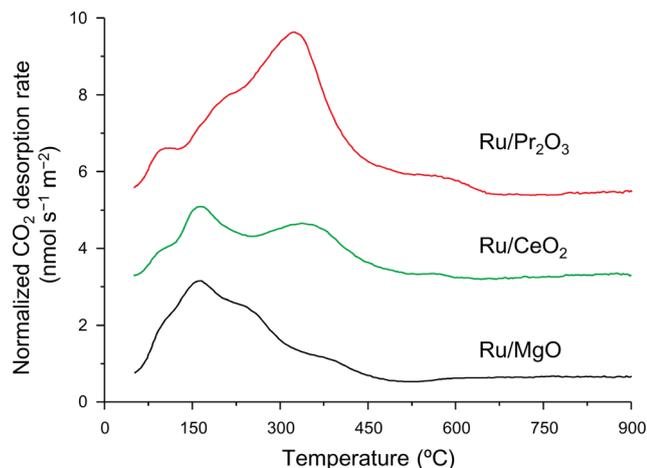
Fig. 5 CO<sub>2</sub>-TPD profiles of supported Ru catalysts. Following H<sub>2</sub> reduction at 400 °C, CO<sub>2</sub> adsorption was carried out at 50 °C. These curves show the difference between the curves shown in Fig. S14† to remove the contribution of CO<sub>2</sub> that remained on the surface of the catalysts even after H<sub>2</sub> pre-treatment.
