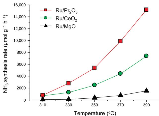
Fig. 2 Rate of  $\text{NH}_3$  synthesis over supported Ru catalysts. Reaction conditions: catalyst, 0.2 g; reactant gas,  $\text{H}_2/\text{N}_2 = 3$  with a flow rate of 60  $\text{mL min}^{-1}$ ; pressure, 0.9 MPa.
