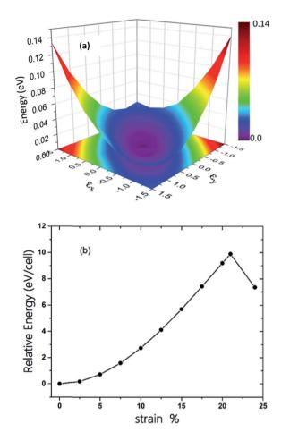
Fig. 3 (a) The three-dimensional surface plots of strain energy *versus* uniaxial strain. (b) Energy of  $C_2S_3N_6$  monolayer as a function of uniform biaxial strain.
