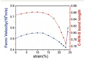
Fig. 6 The Fermi velocities of the  $C_2X_3N_6$  monolayer and the ratio of C-N bonds vs. N-S bonds under uniform biaxial strains. Fermi velocities is blue solid lines and ration of bonds is red solid lines
