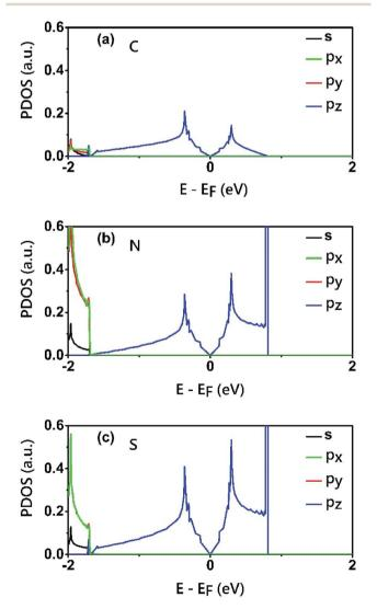
Fig. 5 Electron density of states (PDOS) projected onto the atomic orbitals (s,  $p_x$ ,  $p_y$  and  $p_z$ ) of (a) C (b) N and (c) S atoms of the  $C_2S_3N_6$  monolayer. The energy at the Fermi level was set to zero.
