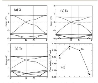
(a-c) Electronic band structures of the C<sub>2</sub>X<sub>3</sub>N<sub>6</sub> monolayer with X = O, Se and Te. The energy at the Fermi level was set to zero. (d) The Fermi velocities of C<sub>2</sub>S<sub>3</sub>N<sub>6</sub> monolayer and its analogs at the equilibrium states
