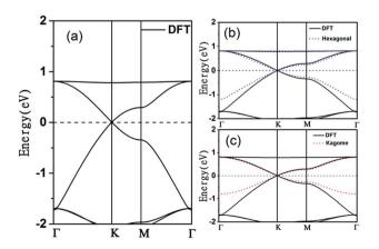
Fig. 4 (a) Electronic band structures of the  $C_2S_3N_6$  monolayer obtained from DFT calculations (b) tight binding Hamiltonian in hexagonal model (hexagonal model is blue dotted lines), (c) tight binding in kagome (kagome model red dotted lines). The energy at the Fermi level was set to zero.
