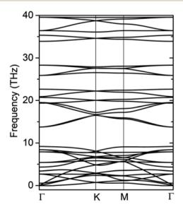
Fig. 2 The phonon spectrum of the  $C_2S_3N_6$  monolayer along the highly-symmetric directions in the BZ.
