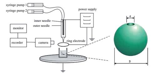
Fig. 14 Experimental setup for the electrohydrodynamic atomization (CEHDA) technique, consisting of a pair of concentric needles. Reproduced from ref. 111 with permission from the American Chemical Society
