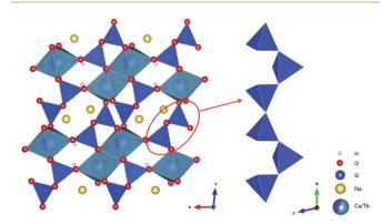
Fig. 2 Polyhedral view of the  $Na_2Tb_{1.08}Ca_{2.92}Si_6O_{18}H_{0.8}$  compound along the *b*-axis and [SiO<sub>4</sub>] tetrahedra single chain.
