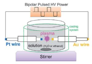
Fig. 14 Image of a synthesis apparatus of a gold/platinum alloy by inliquid plasma using gold and platinum electrodes. Reproduced from Hua and coworkers.<sup>157</sup> Copyright 2013 by Elsevier.
