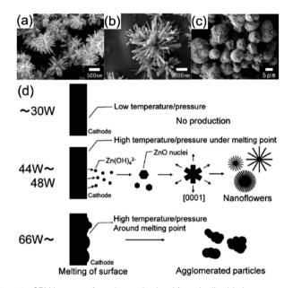
Fig. 15 SEM images of products obtained from in-liquid plasma usage; experimental conditions of  $\rm K_2CO_3$  concentration, and discharge voltage/power are: (a) 1.0 M, 66 V/44 W, (b) 0.5 M, 80 V/48 W, (c) 0.01 M, 200 V/168 W. (d) Schematic processes in the synthesis of ZnO nanoflowers and ZnO aggregates using in-liquid plasma. Modified with permission from ref. 90. Copyright 2011 by Elsevier.
