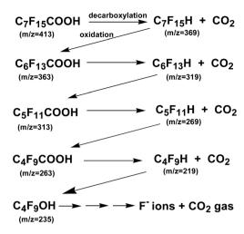
Scheme 1 Sequential loss of  $CF_2$  units from the PFOA perfluorinated acid and decarboxylated intermediates produced during the degradation of PFOA by plasma irradiation for 90 s. Note that loss of  $CF_2$  units after the first decarboxylation step likely occurs by oxidation of the protonated terminal carbon and formation of  $F^-$  ions and  $CO_2$  and so on in the Z-type pathway shown above. From Horikoshi and coworkers. <sup>156</sup> Copyright 2017 by Elsevier.
