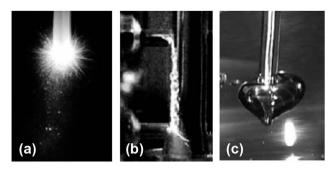
Fig. 19 Method of generating in-liquid plasma for use in water treatment: (a) method of the immersed electrodes in water; (b) method using water flow; (c) method using bubbles. Reproduced from Akiyama *et al.*<sup>220</sup> Copyright 2014 by The Japan Society of Plasma Science and Nuclear Fusion Research.
