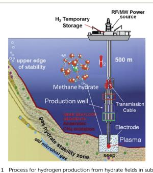
Fig. 1 Process for hydrogen production from hydrate fields in subsea sites using the plasma from the in-liquid method. Reproduced from Rahim and coworkers.<sup>2</sup> Copyright 2015 by Elsevier.
