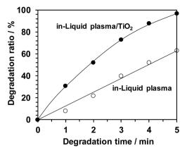
Fig. 21 Decomposition of methylene blue in aqueous solution by inliquid plasma alone and in combination with photocatalyst TiO<sub>2</sub> particles.<sup>17</sup> Copyright 2017 by S. Horikoshi.
