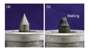
Fig. 9 (a) Photograph of a tungsten pencil-type electrode of an inliquid plasma generator of the microwave type in an unused state; (b) photograph of a tungsten pencil-type electrode after several minutes of generating in-liquid plasma with continuous microwaves. Taken from ref. 17. Copyright 2017 by S. Horikoshi.
