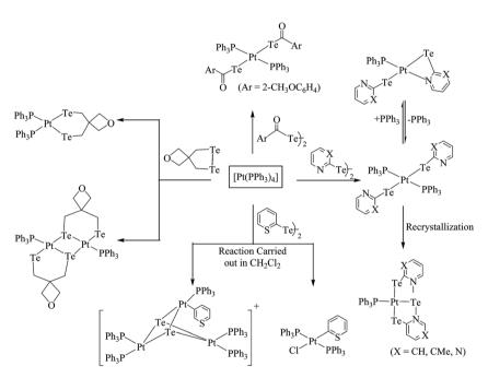
Scheme 16 Oxidative addition reactions of [Pt(PPh<sub>3</sub>)<sub>4</sub>] with various diaryl ditellurides.
