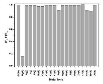
Fig. 3 The quenching of the fluorescence intensity of the GQDs by different metal ions. All the cation concentrations were  $100 \mu M$ . F and  $F_0$  are the emission intensities of the GQDs at  $460 \mu$  nm in the presence and absence of the metal ions.
