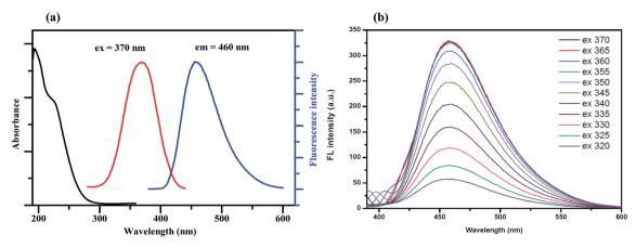
Fig. 1 (a) The absorption (black line), fluorescence excitation (red line) and fluorescence emission (blue line) spectra of the GQDs and (b) the fluorescence spectra of the GQDs at different excitation wavelengths.
