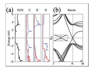
Fig. 3 (a) Total DOS for a graphene layer on h-BN and the projected density of states for C, B and N on the p states in plane (red lines) and out of plane (blue lines), and (b) respective band structure plot of graphene on h-BN, indicating gap opening. Reproduced with permission.43 © 2007 American Physical Society.
