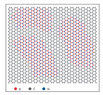
Fig. 25 Atomic model of h-BNC film showing hybridized h-BN and graphene domains. Reproduced with permission.<sup>279</sup> © 2010 Nature Publishing Group
