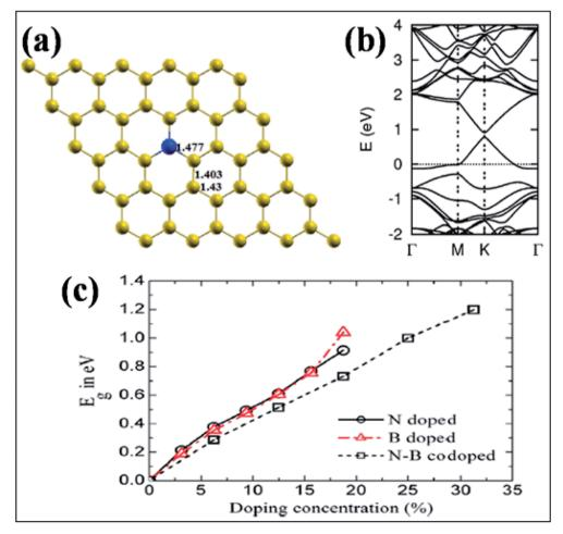
Fig. 14 (a) Substitution of B (blue ball) in graphene. (b) Band structure of a single B-substituted graphene sheet. Reproduced with permission.  $^{159}$  © 2013 Royal Society of Chemistry. (c) Variation of  $E_g$  with N, B, and N-B pair doping concentrations. Reproduced with permission.  $^{164}$  © 2014 Elsevier.
