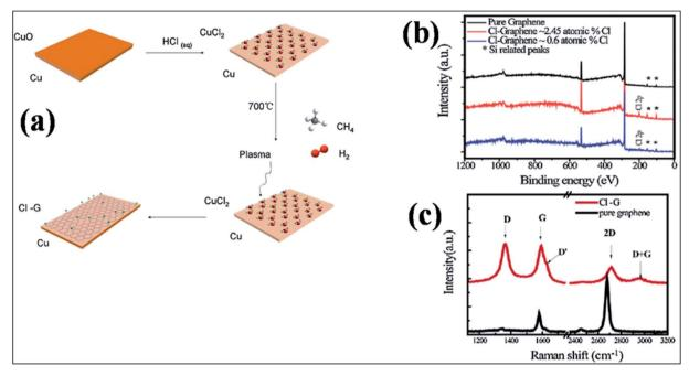
Fig. 12 (a) Schematic representation of the one-step synthesis of chlorinated mono-layer graphene: (b) XPS plots of CCl on  $SiO_2$  compared with that of pure graphene. (c) Raman spectra of graphene (black lines) and CCl (red lines) grown on  $SiO_2$  substrate. Reproduced with permission.<sup>151</sup> © 2015 Elsevier.
