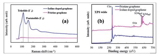
Fig. 9 (a) Raman spectral plot displaying the formation of  $I_3^-$  and  $I_5^-$  in the structure of graphene. (b) XPS spectra of pristine and iodine-doped graphene films. Reproduced with permission. <sup>117</sup> © 2011 Royal Society of Chemistry.
