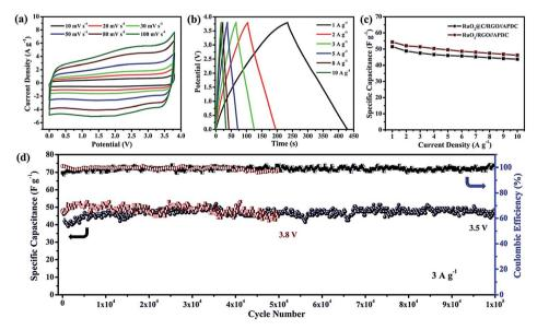
Fig. 15 (a) Cyclic voltammetry (CV) curves and (b) galvanostatic charge/discharge (GCD) curves of the RuO<sub>2</sub>@C/rGO-based ASC. (c) Specific capacitances of the  $RuO_2$ @C/rGO and  $RuO_2$ /rGO-based ASC. (d) Cycling stability and coulombic efficiency of the  $RuO_2$ @C/rGO-based ASC. Reprinted with permission from ref. 118. Copyright 2016 Royal Society of Chemistry.
