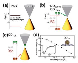
Fig. 8 Schematic illustration of the energy states (a) before depositing QDs on graphene, (b) after depositing QD $_{P2000}$  and QD $_{P500}$  on graphene and (c) after depositing QD $_{TGL}$  on graphene. (d) Photoresponsivity as a function of the incident light power of the QD $_{TGL}$ /GR transistor device. The bottom left inset shows photoresponsivity as a function of gate voltage ( $V_g$ ). Reprinted with an Open Access from ref. 59. Published by WILEY-VCH Verlag Gmbh & Co. KGaA, 2015.
