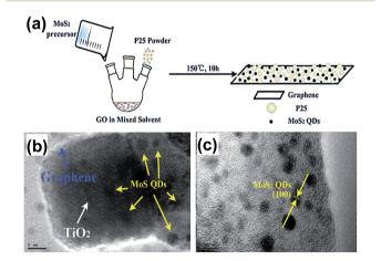
Fig. 4 (a) Schematic demonstration of the fabrication of the  $MoS_2$  QDs-graphene- $TiO_2$  composite. (b) HRTEM image of the  $MoS_2$  QDs-graphene- $TiO_2$  composite. (c) HRTEM image of the  $MoS_2$  QDs-graphene hybrid. Reprinted with permission from ref. 53. Copyright 2015 Royal Society of Chemistry.
