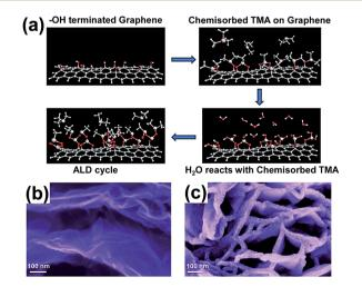
Fig. 5 (a) Schematic diagram of ALD reaction. SEM images of the ZnO QDs/GR composite at 15 ALD cycles (b) and 50 ALD cycles (c). Reprinted with permission from ref. 28. Copyright 2014 Royal Society of Chemistry.
