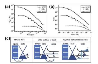
Fig. 12 Photoresponsivity ( $R_{Pn}$ ) (a) and photocurrent gain (b) as a function of applied power for different substrates. (c) Schematic energy band diagrams for different devices and conditions. Reprinted with permission from ref. 92. Copyright 2015 WILEY-VCH Verlag GmbH & Co. KGaA.
