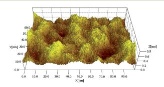
Fig. 1 Image of a single-layer graphene film.<sup>22</sup>
