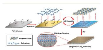
Fig. 8 Schematic of fabrication of polycation/GO NF membrane on PAN substrate via LBL self-assembly.  $^{69}$
