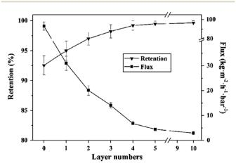
Fig. 9 Effect of layer numbers on separation performance of PDDA/ GO membrane.<sup>69</sup>
