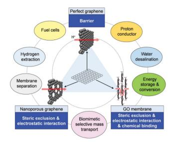
Fig. 4 Schematic illustrating the structure of graphene, NG and GO membrane, the mechanism for selective mass transmembrane transport and possible uses.<sup>52</sup>
