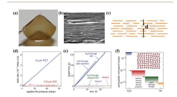
Fig. 5 (a) Photograph of a 1  $\mu$ m-thick GO film; (b) SEM of the film's cross-section; (c) schematic view for possible permeation; (d) He-leak measurements for a GO membrane and a reference PET film; (e) weight loss for a container sealed with a GO film; (f) permeability of GO with respect to water and various small molecules. 52,53
