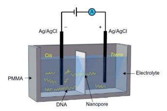
Fig. 1 Schematic view of the NP-based experimental setup. The two chambers (cis and trans) are separated by a membrane, which is usually either biological or solid-state. A nanopore, which was embedded/fabricated into the membrane, acts as the single channel connecting the two chambers. DNA is added to the cis side. Under the electrophoretic force exerted by applied voltage, DNA strands translocate through the NP to the trans chamber, creating characteristic current blockages.2
