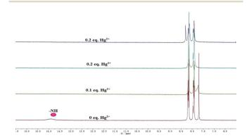
Fig. 7 Partial 1H NMR spectra of Z-3 in DMSO-d $_6$  with different concentrations of  ${\rm Hg}^{2+}$ .
