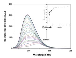
Fluorescence spectra of Z-3 with different concentrations of  $Hg^{2+}$  in DMSO/ $H_2O$  (v/v, 3:2; buffered with HEPES, pH = 7.20) solutions. Insert: plot of fluorescence intensity vs. concentration of  $Hg^{2+}$  in the range of 0 to 63.06 equiv. ( $\lambda_{ex} = 400$  nm).
