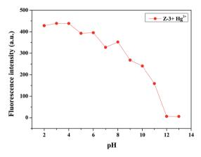
Fig. 4 Fluorescence intensity ( $\lambda_{ex}=400$  nm and  $\lambda_{em}=496$  nm) of the Z-3 + Hg<sup>2+</sup> complex at various pH values in DMSO/H<sub>2</sub>O (v/v, 3:2; buffered with HEPES, pH = 7.20) solution.
