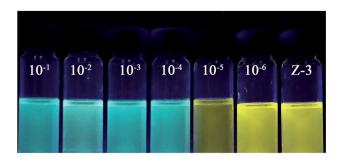
Fig. 6 Naked-eyes detection limit under UV lamp at 365 nm.from left to right, the concentration of  ${\rm Hg^{2+}}$  is  $10^{-1}$  M,  $10^{-2}$  M,  $10^{-3}$  M,  $10^{-4}$  M,  $10^{-5}$  M,  $10^{-6}$  and 0 M.
