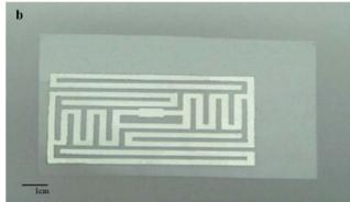
Fig. 25 (a) Photograph of inkjet printed silver patterns on PET substrate showing the metallic luster. (b) Inkjet printed silver ink based RFID antenna. [Reprinted with permission from ref. 120 Copyright © Elsevier.1
