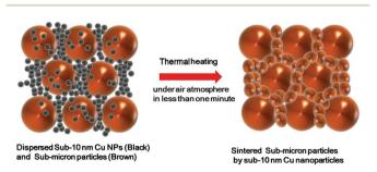
Fig. 30 Schematic illustration of the sintering mechanism of the copper-based composite inks. [Reprinted with permission from ref. 269 Copyright © American Chemical Society.]
