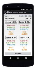
Fig. 23 (Left) Photographs showing both sides of the flexible multigas RFID sensing tag. (Right) A smartphone showing multigas sensing using the Android<sup>TM</sup> application. [Reprinted with permission from ref. 241 Copyright © American Chemical Society.]
