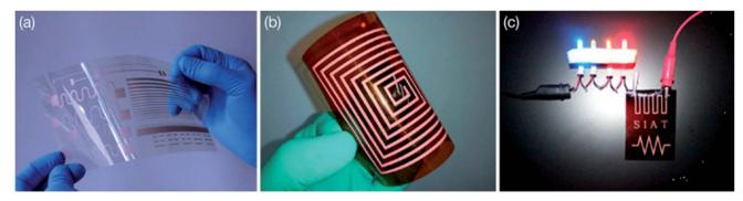
Fig. 31 (a) Photograph of inkjet-printed highly conductive copper patterns on a flexible poly(ethylene naphthalate) (PEN) substrate after plasma treatment. [Reprinted with permission from ref. 271 Copyright © American Chemical Society.] (b) Photograph of the copper-conductive-ink-based printed pattern on a flexible polyimide substrate. (c) Lighted LED device connected with the copper-printed circuit board. [Reprinted with permission from ref. 272 Copyright © American Chemical Society.]
