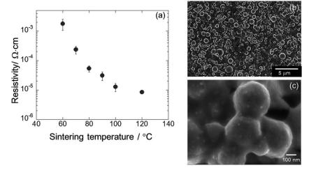
Fig. 29 (a) Change in electrical resistivity of Cu films as a function of sintering temperature. (b, c) SEM images of the sintered Cu films prepared after sintering at 80 °C. [Reprinted with permission from ref. 269 Copyright © American Chemical Society.]
