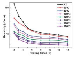
Fig. 20 (Left) Particle size distribution of silver nanoparticle (AgNP) ink with an average AgNP size of 30–50 nm. Insert shows the TEM image of AgNPs imparted in the silver ink formulation. (Right) Electrical resistivity of AgNPs conductive patterns printed on photo-paper as a function of the number of printing cycles (N) after heating from room temperature to 180 °C. [Reprinted with permission from ref. 233 Copyright © The Royal Society of Chemistry.]
