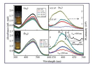
Fig. 21 Photocatalytic and photoluminescence spectra of anataseand rutile-TiO<sub>2</sub> nanoparticles. UV-Vis spectra of the photodegradation of methyl orange dye by anatase (a20) and rutile (b20), respectively, at various time intervals. (a21), and (b21) show the PL characteristics of anatase and rutile, respectively at  $\lambda_{ex} = 300$  nm.<sup>23</sup> Reprinted with permission from ref. 23. Copyright 2016. Elsevier.
