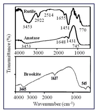
Fig. 19 FT-IR spectra of brookite-, anatase- and rutile- $TiO_2$  nanoparticles. <sup>23,301</sup> Reprinted with permission from ref. 23. Copyright 2016. Elsevier and ref. 301. Copyright 2000. Springer.
