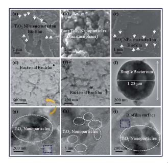
**Fig. 25** (a)–(c) SEM micrographs of TiO<sub>2</sub> nanoparticles (700 μg ml<sup>-1</sup>) interaction with *Enterobacter* sp. for 72 h incubation, TEM images of (d)–(f) bare *Enterobacter* sp. and (g)–(i) interaction of TiO<sub>2</sub> nanoparticles with bacterial biofilm. Blue squares (in (g) and (i)) represent a ruptured biofilm.<sup>51</sup> Reprinted with permission from ref. 51. Copyright 2017. Taylor and Francis.
