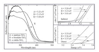
Fig. 20 Optical characteristics: (a) UV-Vis reflectance spectra, (b) optical band gap evaluation of multiphase TiO<sub>2</sub> nanoparticles, where the symbols A, B and R correspond to anatase-, brookite and rutile-TiO<sub>2</sub>.<sup>289</sup> Reprinted with permission from ref. 289.
