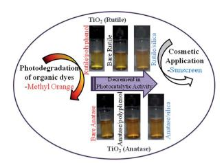
Scheme 4 Pictorial representation of the photodegradation of methyl orange by  $TiO_2$  nanoparticles.<sup>23</sup> Reprinted with permission from ref. 23. Copyright 2016. Elsevier.
