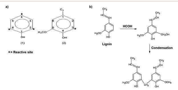
Fig. 10 (a) (1) Phenol structure with three reactive sites, 2-, 4- and 6-position, and (2) typical lignin structure with 1 reactive site, 3-position. (b) Crosslinking between lignin and formaldehyde (reproduced from ref. 85 with permission from Elsevier Ltd).
