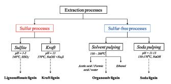
Fig. 2 Different extraction processes to separate lignin from lignocellulosic biomass and corresponding productions of technical lignin (reproduced from ref. 33 with permission from Elsevier Ltd).
