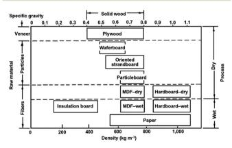
Fig. 1 Classification of wood-based panels.<sup>17</sup>
