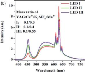
Fig. 8 (a) Concentration dependent emission spectra of  $K_3AlF_6:Mn^{4+}$ . (b) Electroluminescence spectra of prototype LEDs, employing  $K_3AlF_6:Mn^{4+}$  as the red converter component, commercial yellow YAG:Ce<sup>3+</sup> and a blue InGaN chip at a 40 mA drive current.<sup>42</sup>
