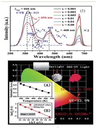
Fig. 6 (1) PL spectra of K<sub>2</sub>BaGe<sub>8</sub>O<sub>18</sub>:Mn<sup>4+</sup> with different concentrations, and PL excitation spectra of the K<sub>2</sub>BaGe<sub>8</sub>O<sub>18</sub>:0.002Mn<sup>4+</sup> sample monitored at 666 nm and 654 nm. (2) Chromatic CIE coordinates, quantum yields and variation of emission intensity depending on the temperature of the representative K2BaGe8O18:Mn4+.32
