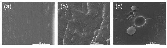
Fig. 2 SEM images for WPU films (a), BWPU film (b), and GWPU film (c).49
