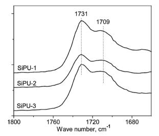
Fig. 8 FT-IR spectra of urethane C=O stretching region of PDMS-modified WPU (reproduced from ref. 50 with permission from the Royal Society of Chemistry). The PDMS content in soft segments for SiPU-1, SiPU-2, and SiPU-3 is 50%, 60%, and 67%, respectively.
