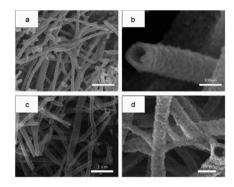
Fig. 20 (a) Low- and (b) high-magnification SEM images of  $In_2O_3$  and (c) low- and (d) high-magnification SEM images of  $Fe_2O_3-In_2O_3$  nanotubes after annealing at 500 °C (this figure has been adapted from ref. 73 with permission from Elsevier).
