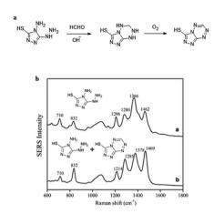
Fig. 14 (a) Derivative reaction of FA and AHMT under alkaline conditions. (b) SERS spectra of 500  $\mu$ L (a) AHMT in deionized water and (b) AHMT–MTT mixture in HCHO solution (this figure has been reproduced from ref. 70 with permission from Springer).
