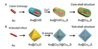
Fig. 1 Scheme of synthesizing the  $Au-Cu_{2-x}S$  hybrid based on the template method.<sup>49,63</sup> (A) Reprinted with permission from ref. 63. Copyright 2016 Wiley-VCH Verlag & Co. KGaA. (B) Reprinted with permission from ref. 49. Copyright 2016 American Chemical Society.
