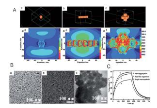
**Fig. 6** (A) Simulation of the LSPR for (a, d) single nanoparticles, (b, e) rod-like self-assembly, and (c, f) nanosuperlattices, respectively. (B) TEM images of the prepared nanocomposites. (C) Temperature profiles of obtained nanocomposites irradiated with and without laser. <sup>86</sup> Reprinted with permission from ref. 86. Copyright 2015 Wiley-VCH Verlag & Co. KGaA.
