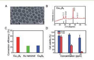
Fig. 9 (A) TEM image and (B) XRD of the obtained  $Cu_{7.2}S_4$  NPs. (C) Comparison of PTCE for  $Cu_{7.2}S_4$ , gold nanorod and  $Cu_9S_5$  under the irradiation of a 980 nm laser, respectively. (D) Cell viability after treatment with  $Cu_{7.2}S_4$  NPs at different concentration before and after the irradiation of the 980 nm laser.<sup>60</sup> Reprinted with permission from ref. 60. Copyright 2014 Royal Society of Chemistry.
