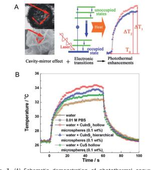
Fig. 3 (A) Schematic demonstration of photothermal conversion enhancement and temperature elevation based on the cavity-mirror effect and interband transitions. (B) Temperature elevation of water, PBS and different superstructures under laser irradiation. <sup>76</sup> Reprinted with permission from ref. 76. Copyright 2013 American Chemical Society.
