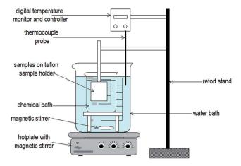
Fig. 8 Experimental setup used for chemical bath deposition. 68
