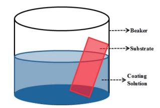
Fig. 14 Schematic of dip coating technique.
