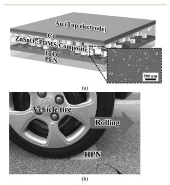
Fig. 18 (a) Schematic diagram of ZnSnO<sub>3</sub>:PDMS-based flexible hybrid PENG. (b) Experimental setup used for the generation of power from the hybrid PENG under a rolling vehicle tire.200
