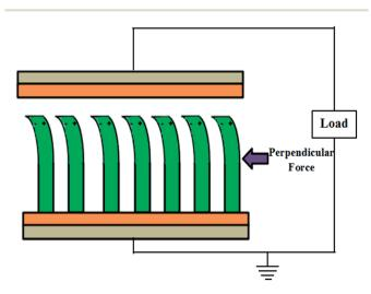
Fig. 2 Schematic of PENG after the application of a force perpendicularly to the NG axis.
