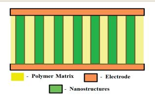
Fig. 5 Schematic diagram of NEG.
