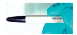
Fig. 22 Fully rollable graphene-based NG. 103
