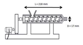
Fig. 7 Representation of a single-screw extruder.
