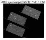
Fig. 6 Possible decrease of the porosity in polycaprolactone reinforced with natural hemp fibers after an injection process (porosity measured by scanning electron microscopy and image analysis).
