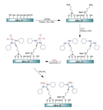
Fig. 23 Preparation of SBA-15/1,3-DCG/Pd. Reprinted from ref. 121 with permission of Royal Society of Chemistry.
