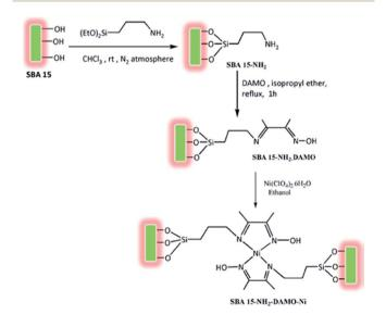
Fig. 7 Route to synthesize functionalized SBA-15 supported nickel(II)oxime-imine catalysts. Reprinted from ref. 99 with permission of Elsevier
