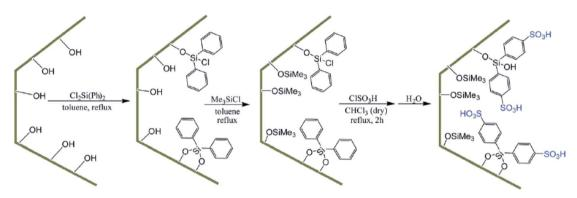
Fig. 36 Preparation of SBA-15-Ph-SO<sub>3</sub>H. Reprinted from ref. 158 with permission of Royal Society of Chemistry.
