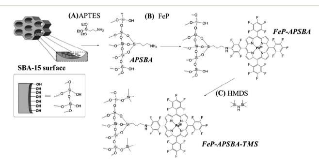
Fig. 21 (A) Preparation of the hybrid material APSBA from the starting SBA-15 structure; (B) FeP immobilization on the hybrid APSBA, to give FeP-APSBA; and (C) silylation of the FeP-APSBA surface with HMDS, to yield FeP-APSBA-TMS. Reprinted from ref. 119 with permission of Royal Society of Chemistry.
