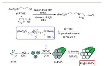
Fig. 16 Procedures for the synthesis of the Pd@IL-PMO. Reprinted from ref. 111 with permission of Elsevier.
