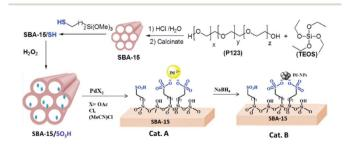
Fig. 24 Schematic representation of the catalysts preparation. Reprinted from ref. 122 with permission of Elsevier.
