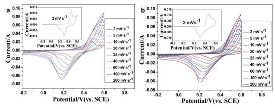
Fig. 5 CV curves of the Mn-LMOF electrode at sweep rates from 2 to 200 mV s $^{-1}$  in (a) 1 M KOH and (b) 1 M LiOH solution.
