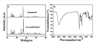
Fig. 1 (a) XRD pattern of as-synthesized Mn-LMOF and the simulated pattern based on the crystal data of Mn-LMOF (b) FT-IR spectrum of the Mn-LMOF.
