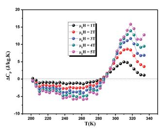
Fig. 4 Change of specific heat of the sample as a function of temperature at different magnetic fields for x = 0.05.
