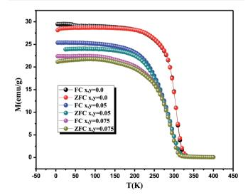
**Fig. 1** Temperature dependences of ZFC and FC magnetization for  $La_{0.7}Ca_{0.1}Pb_{0.2}Mn_{1-x-y}Al_xSn_yO_3$  (x, y = 0.0, 0.05 and 0.075) compounds under a magnetic field of 0.05 T.
