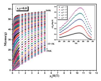
Fig. 2 Magnetic field dependence of magnetization at several temperatures for La $_{0.7}$ Ca $_{0.1}$ Pb $_{0.2}$ Mn $_{1-x-y}$ Al $_x$ Sn $_y$ O $_3$  (x,y=0.0) sample, the inset: temperature dependence of the magnetic entropy change ( $-\Delta S_{\rm M}$ ) at different applied magnetic field change intervals for La $_{0.7}$ Ca $_{0.1}$ Pb $_{0.2}$ Mn $_{1-x-y}$ Al $_x$ Sn $_y$ O $_3$  (x,y=0.05).
