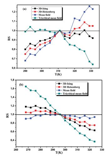
Fig. 7 Relative slope (RS) as a function of temperature of La<sub>0.7</sub>Ca<sub>0.1</sub>- $Pb_{0.2}Mn_{0.9}Al_{0.05}Sn_{0.05}O_{3}$ , (a) for x, y = 0.0 and (b) for x, y = 0.05.
