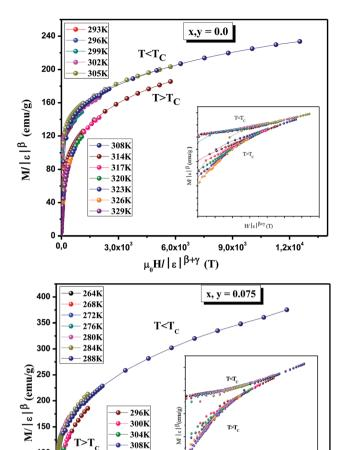
Fig. 12 Scaling plots for  $La_{0.7}Ca_{0.1}Pb_{0.2}Mn_{1-x-y}Al_xSn_yO_3$  (x, y=0.0and 0.075) below and above  $T_{\rm C}$  using  $\beta$  and  $\gamma$  determined by the Kouvel-Fisher method. The insets show the same plots on a log-log scale.
