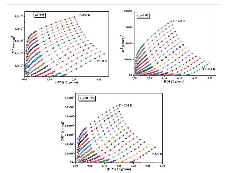
Fig. 5 Arrott plots around  $T_C$  for La<sub>0.7</sub>Ca<sub>0.1</sub>Pb<sub>0.2</sub>Mn<sub>1-x-y</sub>Al<sub>x</sub>Sn<sub>y</sub>O<sub>3</sub> (x, y = 0.0, 0.05 and 0.075) samples. According to the mean field model, values of critical exponents  $\beta = 0.5$  and  $\gamma = 1$  should generate the regular Arrott plots,  $M^2$  vs.  $\mu_0 H/M$ .
