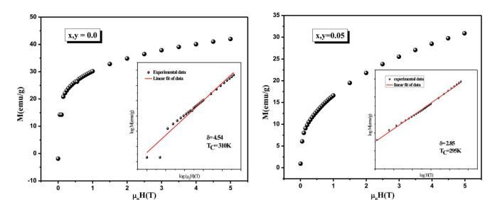
Fig. 10 Critical isotherms of *M versus*  $\mu_0 H$  for La<sub>0.7</sub>Ca<sub>0.1</sub>Pb<sub>0.2</sub>Mn<sub>1-x-y</sub>Al<sub>x</sub>Sn<sub>y</sub>O<sub>3</sub> (x, y = 0.0 and 0.05). The inset: shows the log-log scale for *M versus*  $\mu_0 H$ .
