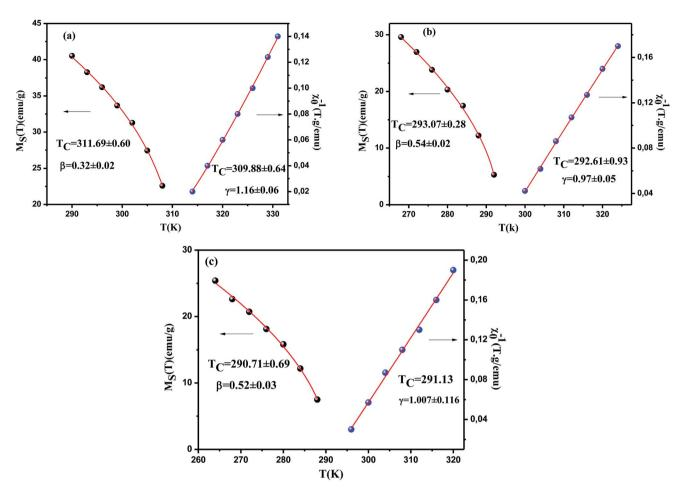
Fig. 8 The spontaneous magnetization  $M_S(T, 0)$  (left) and the inverse initial susceptibility  $\chi_0^{-1}(T)$  (right) as a function of temperature of La<sub>0.7</sub>-Ca<sub>0.1</sub>Pb<sub>0.2</sub>Mn<sub>0.9</sub>Al<sub>0.05</sub>Sn<sub>0.05</sub>O<sub>3</sub>, (a) for x, y = 0.0, (b) for x, y = 0.05 and x, y = 0.075.
