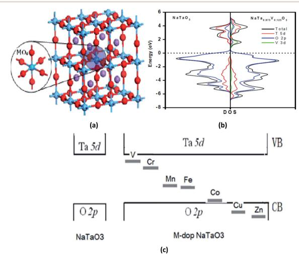
Fig. 6 (a) A supercell of M-doped NaTaO $_3$  2 × 2 × 2 (40-atoms), (b) the total density of states and projected density of states of the pure and Vdoped NaTaO<sub>3</sub>, and (c) intermediate band formation by the d-orbital of the doped metal ions. Reprinted with permission of ref. 184. Copyright 2012 IACSIT Press, Singapore.
