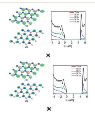
Fig. 7 The plane-wave DFT calculations of the electronic structure of h-BN and h-BCN. The optimized structure of B<sub>16</sub>N<sub>16</sub> with the corresponding valence band (VB)/conduction band (CB) and the corresponding total and ion-decomposed electronic density of states (a and b). Reprinted with permission of ref. 215. Copyright 2015 Macmillan Publishers Limited
