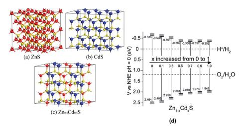
Fig. 8 The supercell models for bulk (a) ZnS (64 atoms) and (b) CdS (64 atoms). The red, yellow, and blue spheres represent the Zn, S, and Cd atoms, respectively. (c) The geometry model for  $Zn_{0.5}Cd_{0.5}S$  and (d) conduction and valence band edge potentials of the  $Zn_{1-x}Cd_xS$  samples (x = 0, 0.1, 0.3, 0.5, 0.7, 0.9, and 1.0). Reprinted with permission of ref. 223. Copyright 2013 American Chemical Society.
