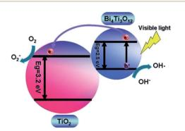
Fig. 3 A schematic showing the energy band structure and electron–hole pair separation in the  $Bi_4Ti_3O_{12}/TiO_2$  heterostructure. Reprinted with permission of ref. 124. Copyright 2011 Royal Society of Chemistry.
