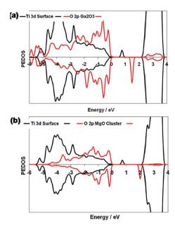
Fig. 4 Ti 3d and O 2p PEDOS of the  $(Ga_2O_3)_2$  and  $(MgO)_4$  clusters for the relaxed triplet excited states of (a)  $Ga_2O_3$ -modified  $TiO_2$  and (b) MgO-modified  $TiO_2$ . The zero of energy is the top of the valence band. Reprinted with permission of ref. 134. Copyright 2012 American Chemical Society.
