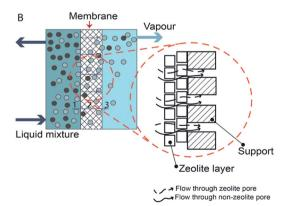
Fig. 1 Schematic of pervaporation process. (A) Type of pervaporation and (B) mechanism of pervaporation process.
