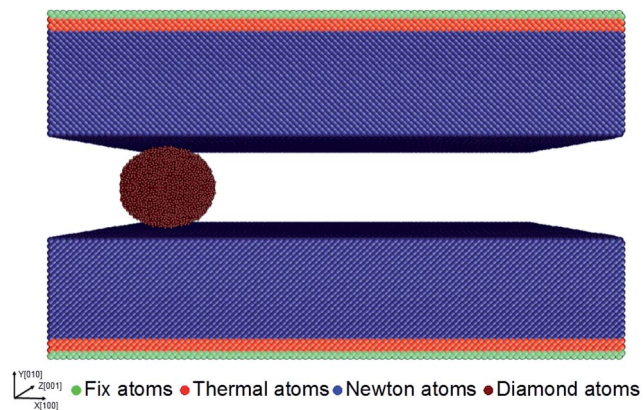
Fig. 2 Schematic of the MD simulation model for three-body abrasion in a vertical cross-section.
