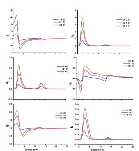
Fig. 8 The real and imaginary parts of dielectric function ( $\varepsilon_1$  and  $\varepsilon_2$ ) (top); real and imaginary parts of conductivity ( $\sigma_1$  and  $\sigma_2$ ) (center) and refractive index (n)/extinction co-efficient (k) (bottom) of nitrogen-doped nanographene NDG compound **1** in three directions, respectively.
