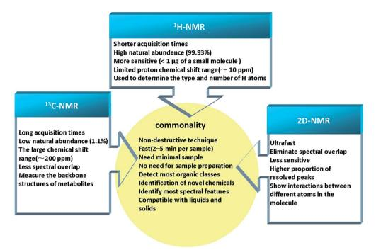
Fig. 2 The commonality and features between <sup>1</sup>H-NMR, <sup>13</sup>C-NMR and 2D-NMR.
