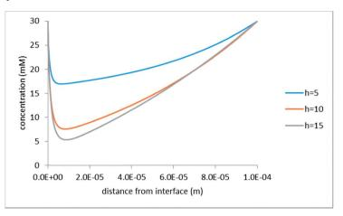
Fig. 8 Concentration distribution along the z-axis at the hole edge;  $\varphi_0 = 200$  mV; the legend indicates half-distance between the hole centers in micrometers.
