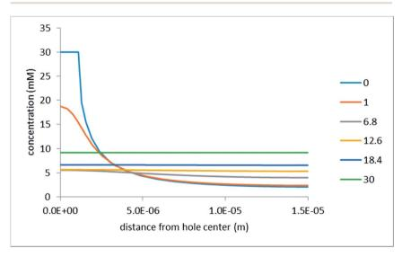
Fig. 6 Salt-concentration profiles in the horizontal direction at various distances (in  $\mu$ m) from the mask/porous-medium interface as indicated in the legend: hole radius 1  $\mu$ m, inter-hole spacing 30  $\mu$ m, voltage drop 200 mV.
