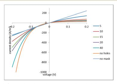
Fig. 10 Current-voltage characteristics; the legend indicates the half-spacing between the holes (in micrometers); the hole radius is  $1 \mu m$ .
