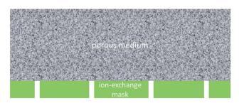
Fig. 1 Sketch of a nano-porous layer sandwiched with a perforated ion-exchange mask (not to scale).
