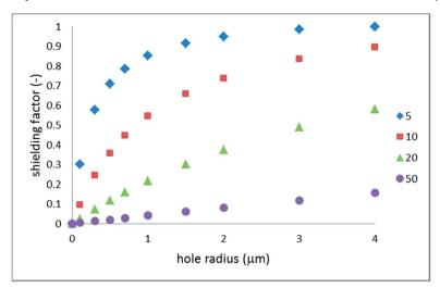
Fig. 3 Hydraulic shielding factor vs. hole radius; the legend indicates the cell size (half-distance between the hole centers) in micrometers.
