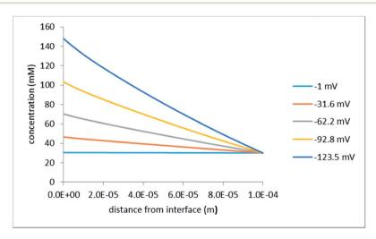
Fig. 9 Concentration distribution along the z-axis at the upper right cell corner (see Fig. 2); the legend indicates the applied voltages; the half-distance between the hole centers is 15  $\mu$ m.
