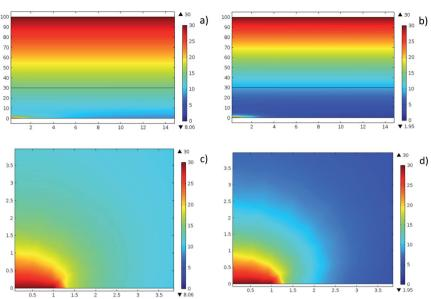
Fig. 5 Salt-concentration distributions in the vertical plane passing through the hole center: hole radius 1 m $\mu$ , cell half-size 15  $\mu$ m; in the upper maps (a, b) the scales along the vertical and horizontal axes are different; the lower maps (c, d) show the magnified vicinity of the hole with the same scaling along both axes. The hole center is in the lower left corner. (a, c)  $\varphi_0=93$  mV; (b, d)  $\varphi_0=200$  mV.
