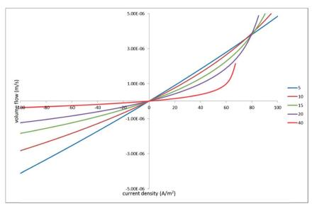
Fig. 12 Volume flux vs. current density; the legend indicates the half-distances between the hole centers in micrometers.
