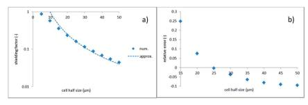
Fig. 4 Shielding factor vs. half inter-hole spacing; hole radius is 1  $\mu$ m; (a) numerics vs. scaling law of eqn (32); (b) relative error of scaling law.
