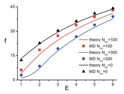
Fig. 3 The dependence of the generated force  $\tilde{f}=fb/k_BT$  on the applied electric field  $\tilde{E}=eEb/k_BT$  for Hertzian springs ( $\gamma=3/2$ ) with  $\tilde{\kappa}=\kappa b\gamma/k_BT=1$  for  $N_{\rm ion}=0$ ,  $N_{\rm ion}=100$  ( $n_{\rm s}=4.6\times10^{-4}$  M), and  $N_{\rm ion}=300$  ( $n_{\rm s}=1.38\times10^{-3}$  M) obtained theoretically and in the MD simulations. The data are shown for L=40b,  $S=50\times50b^2$ ,  $l_0=20b$  and  $N_0=80$ .
