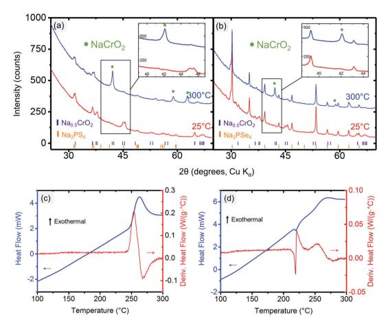
Fig. 6 XRD results for reaction between (a)  $Na_{0.5}CrO_2$  and  $Na_3PS_4$  and (b)  $Na_{0.5}CrO_2$  and  $Na_3PSe_4$  at RT (25 °C) and 300 °C. DSC results for reaction between (c)  $Na_{0.5}CrO_2$  and  $Na_3PSe_4$  and (d)  $Na_{0.5}CrO_2$  and  $Na_3PSe_4$ .
