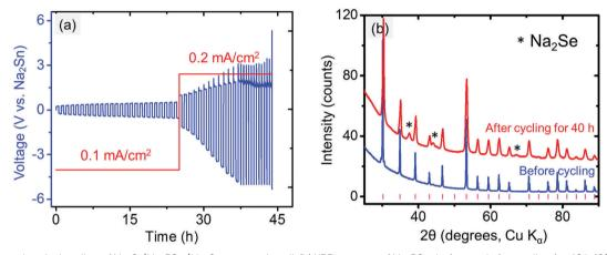
Fig. 9 (a) Electrochemical cycling of  $Na_2Sn|Na_3PSe_4|Na_2Sn$  symmetric cell. (b) XRD patterns of  $Na_3PSe_4$  before and after cycling for 40 h (60 min per cycle); the tick marks indicate  $Na_3PSe_4$  peaks.
