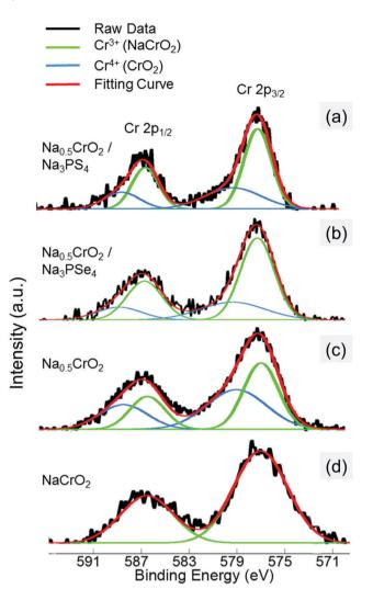
Fig. 7 XPS spectra of Cr 2p from the surfaces of (a) mixture of Na<sub>0.5</sub>CrO<sub>2</sub> and  $Na_3PS_4$  at RT (25 °C), (b) mixture of  $Na_{0.5}CrO_2$  and  $Na_3PSe_4$  at RT (25 °C), (c) Na<sub>0.5</sub>CrO<sub>2</sub>, and (d) NaCrO<sub>2</sub>.
