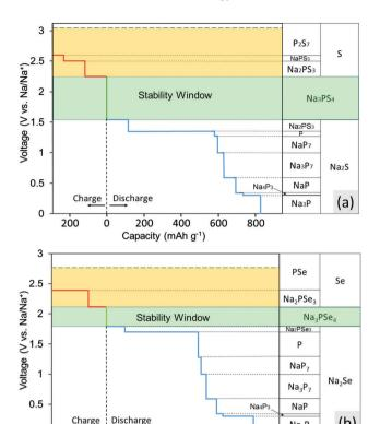
Fig. 2 Calculated stability window and decomposition products for (a) Na<sub>3</sub>PS<sub>4</sub> and (b) Na<sub>3</sub>PSe<sub>4</sub>. The green shaded region is the thermodynamically stable voltage window, and the yellow shaded region is the additional voltage range that could be kinetically stabilized.
